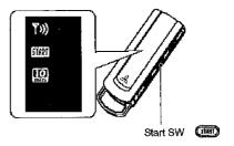
When the wireless communication between the transmitter and the receiver unit is correctly done, the engine starts.
