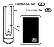
Push Function SW and Switch Unlock SW at the same time until buzzer sounds.
