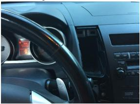
9. Pry on the bottom of the dash cover, then tug the rest off, it should look like this. Also, pull the plug for the info button.
