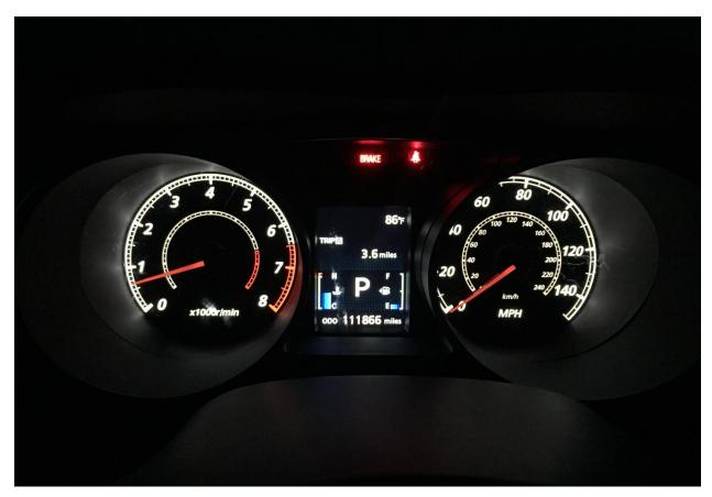
NOTE: If the check engine light is on, you probably turned on the car with the cluster unplugged. Just get any normal code reader for your OBD port and erase the code, or perhaps try unplugging the battery for a minute and reattach.
