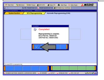
The Daytime Running Lights and both the engine and condenser fans will automatically be turned on during reprogramming. Care should be taken to insure nothing gets caught in the moving blades. The radio will be turned off and you will also hear a chime in the interior for a short period of time. These are normal conditions.
