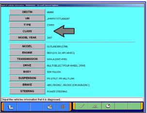
h. If it was not completed automatically, input the vehicle class. Click on the CLASS button, select the appropriate class from the menu (below left) and then click the check mark at the bottom of the page. Vehicle class can be found on the Vehicle Information Code Plate riveted to the base of the RH b-pillar (see photo below right). The class is part of the model code.
