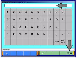
g. Click on the icon in the lower RH corner of the screen to have the MUT III automatically read the VIN.
